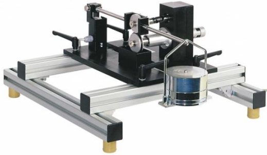
Fig 1: TM 260.01 Rolling and Sliding Disc Tribometer [12]. This Tribometer consists of two friction disc that are in contact, driven by a gearbox unit clamped with a motor. A lubricant tank that contains the nanolubricant is placed directly below the friction discs and a load mechanism is used to vary the load applied on the friction. The rolling and sliding disc Tribometer is used with a control unit having a motor connected to its rear socket. The control unit is used to regulate the speed of the motor clamped to the gearbox unit and display the friction force in the contact between the two discs.
