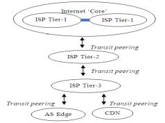
Figure 1. above shows traditional structure i.e. hierarchical topology of Internet in which lower level Providers pays Transit Providers to route traffic.
