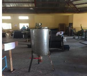
Figure 4: The developed paint production machine 2.5 Performance Evaluation of the Paint Production Machine
