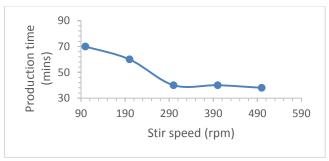
Figure 7: Effect of Stir Speed on Production time
