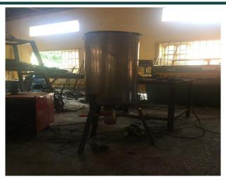
Figure 3: The paint mixer at the developmental stage The developed machine is shown in Figure
