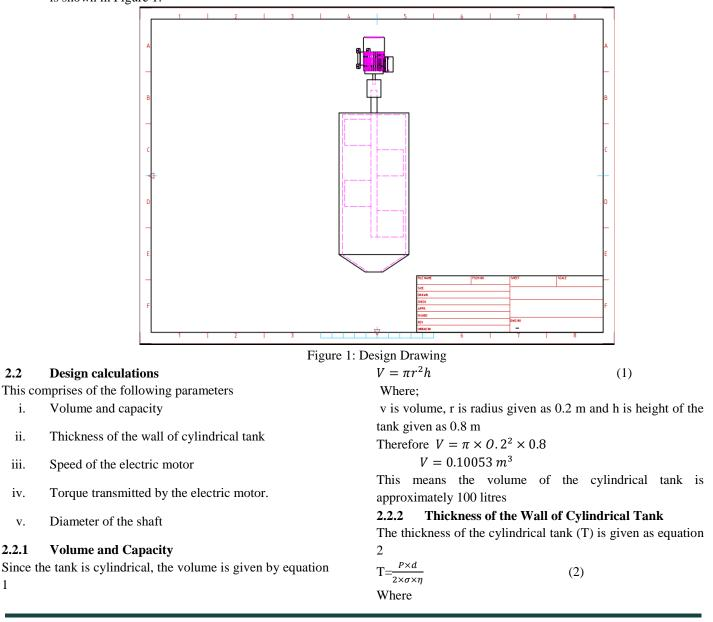
P is the internal pressure  $(0.5 N/mm^2)$ ;  $\eta$  is the joint efficiency (0.95);  $\sigma$  is the circumference stress (5.26  $N/mm^2$ )
