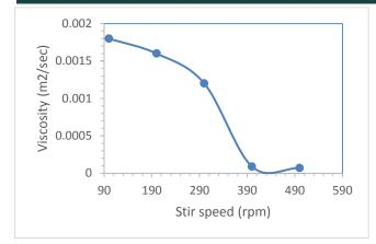
Figure 6: Effect of stir speed on paint viscosity The effect of stir speed on production time was also studied and presented in Table 4.
