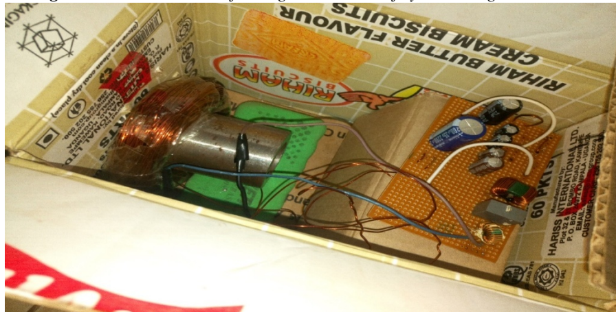
Figure 7. Shows the transmitter circuit of the project system.
