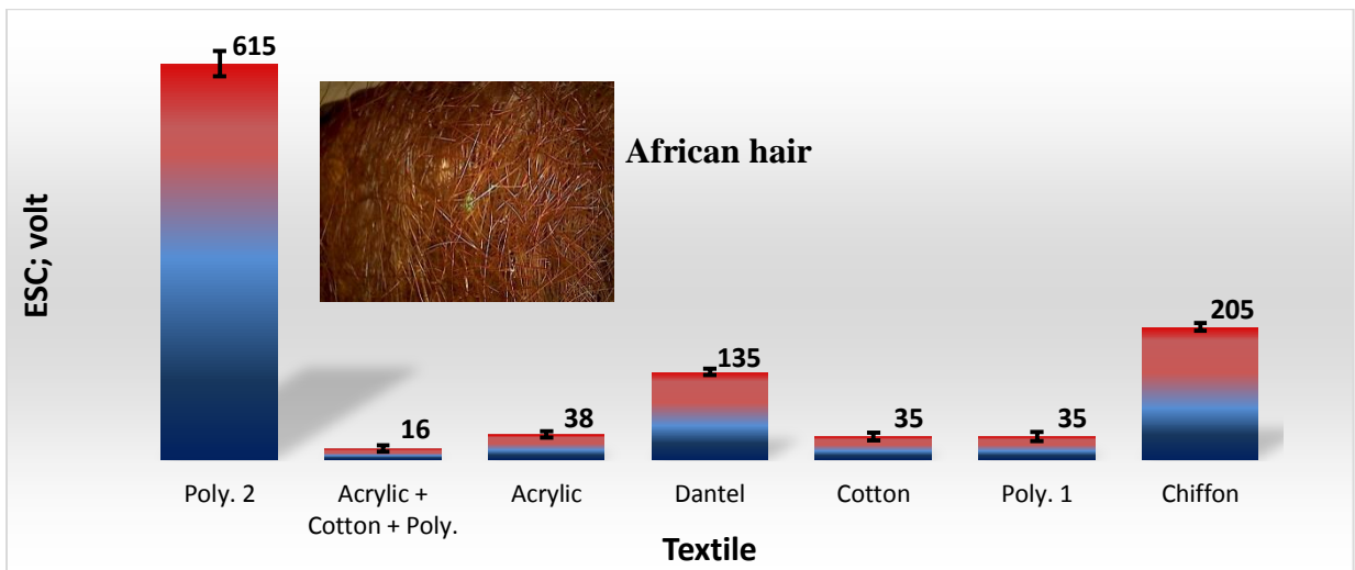
Fig. 6. ESC generated from sliding of African hair against different types of textiles.
