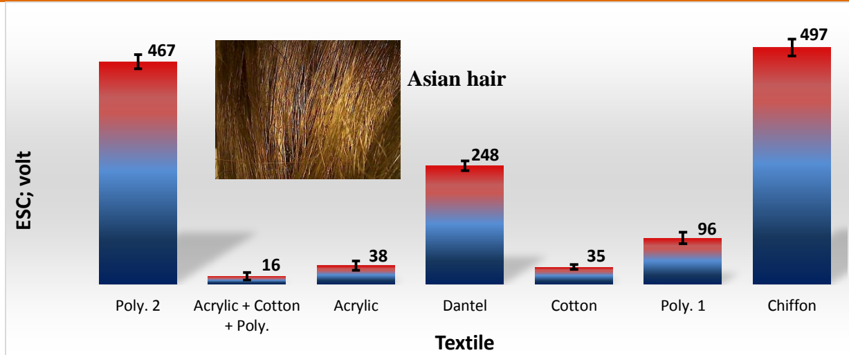
Fig. 8. ESC generated from sliding of Asian hair against different types of textiles.
