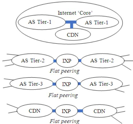
Figure. 2 above shows flattening peering of Internet.
