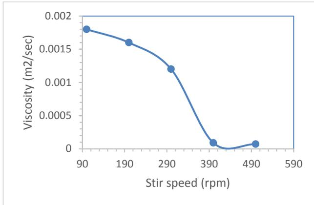
Figure 6: Effect of stir speed on paint viscosity
