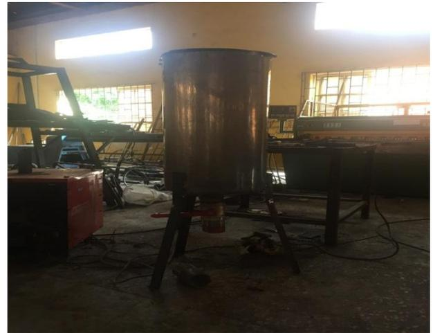
Figure 3: The paint mixer at the developmental stage
