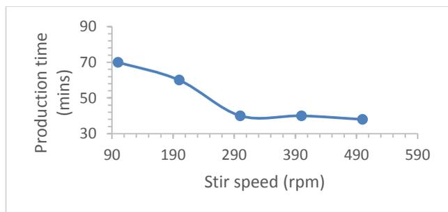
Figure 7: Effect of Stir Speed on Production time
