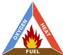
The Triangle of fire consists of (Fuel-Heat – Oxygen); eliminating one side of the triangle prevents the occurrences
