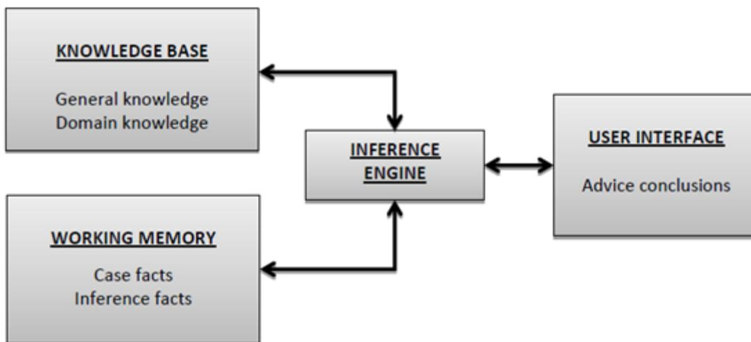
Figure 1: The structure of a knowledge-based expert system
