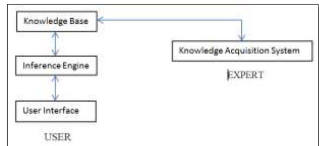
Figure 1: Main components of an Expert System [8]
