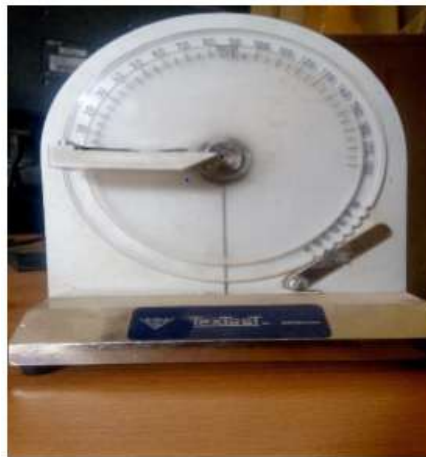
Figure 3: the ' Shirley' crease recovery instrument (CRA)
