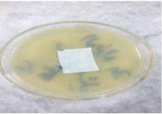
Fig (6.2): (A-ZnO) treated fabric with (E.coli before washing)
