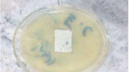
Fig (6.4): (A-ZnO) Treated fabric with E- coli after washing
