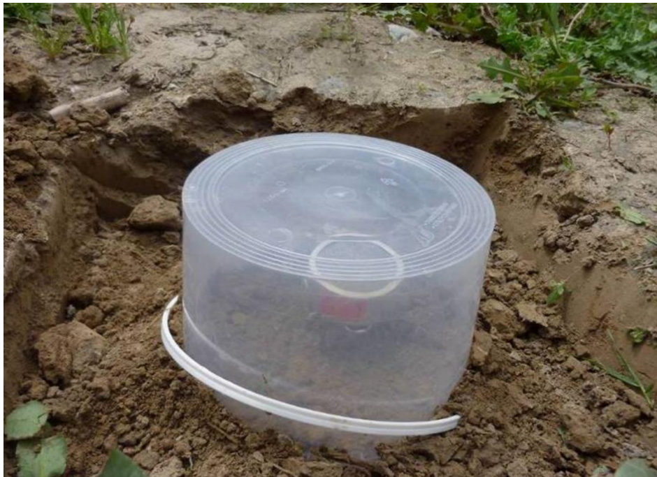
Fig. 1. Radon absorber, covered with a plastic storage chamber to determine the RFD (radon flux density)
