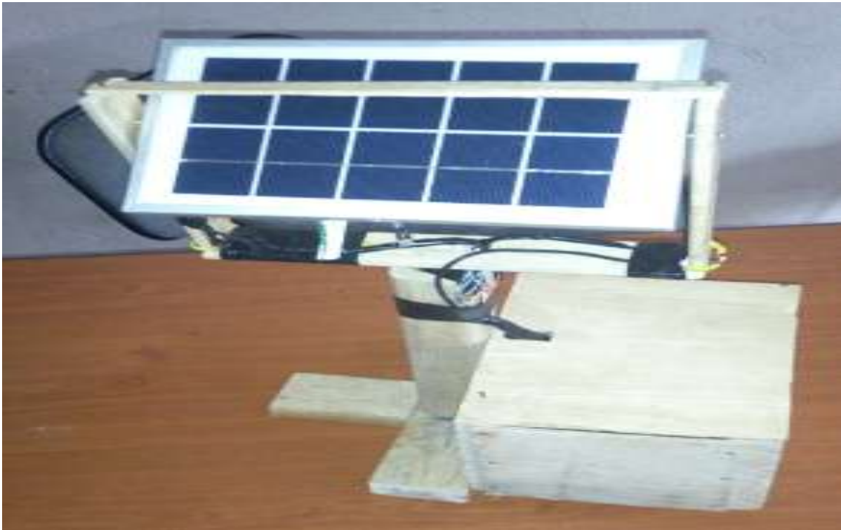
Figure 5: Dual axis tracking system
