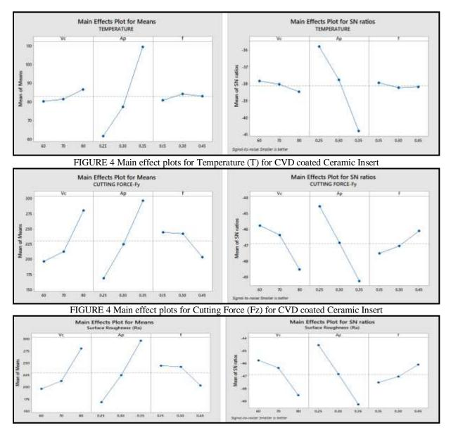
FIGURE 4 Main effect plots for surface roughness for CVD coated carbide Insert
