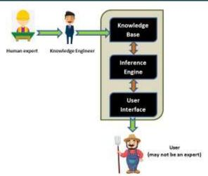
Figure 2: Expert System Architecture
