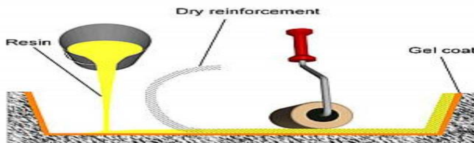
Figure 1: hand lay-up method
