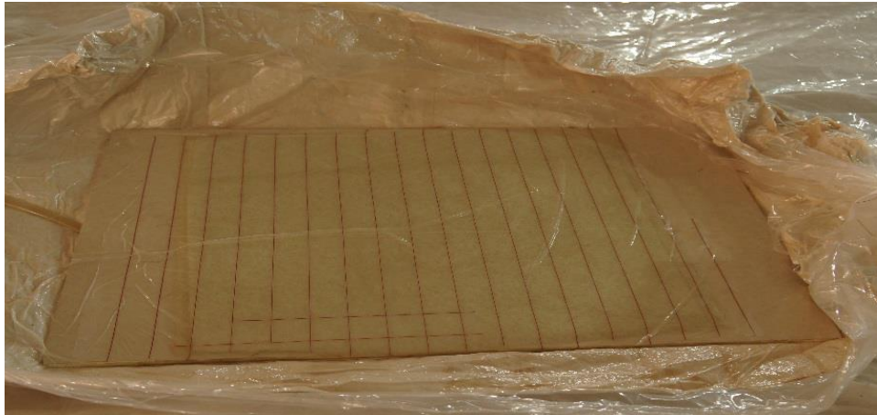
Figure 2: vacuum bagging method
