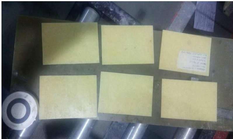
Figure 3: Specimens preparation for impact drop weight
