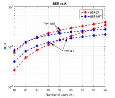
Figure 3: Diagram showing the relationship between BER and the number of users K when M=100.
