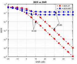
Figure 2b: Diagram showing the relationship between BER and SNR when M=100
