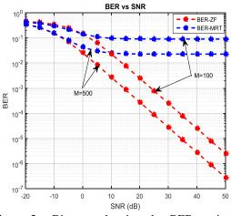
Figure 2a: Diagram showing the BER against SNR when K=50
