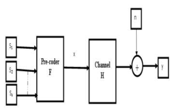
Figure 1: Diagram showing downlink massive MIMO.
