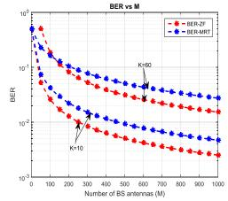
Figure 5: Showing the relationship between BER and the number of BS antennas when Pd=0dB
