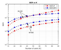
Figure 4: Diagram showing the relationship between BER and the number of users K at Pd=0dB
