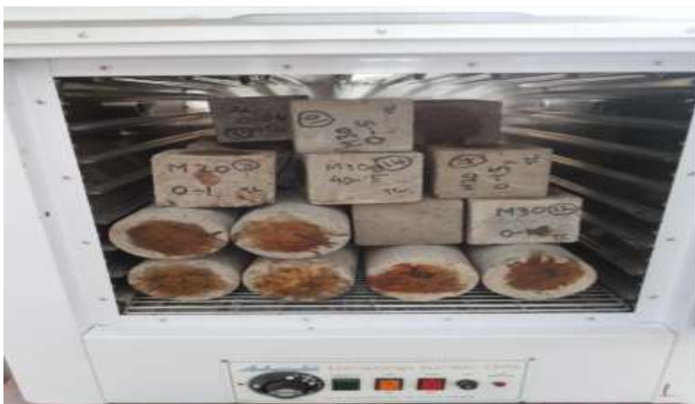
Figure 4: Concrete Specimens Subjected to Elevated Temperature
