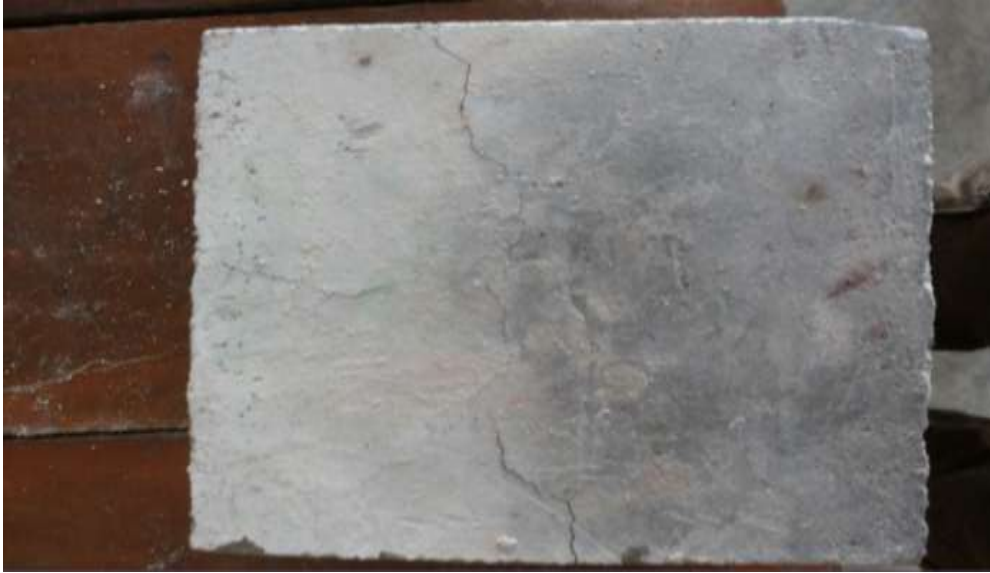
Figure 5: Concrete Specimens after Exposed to 600°C Temperature
