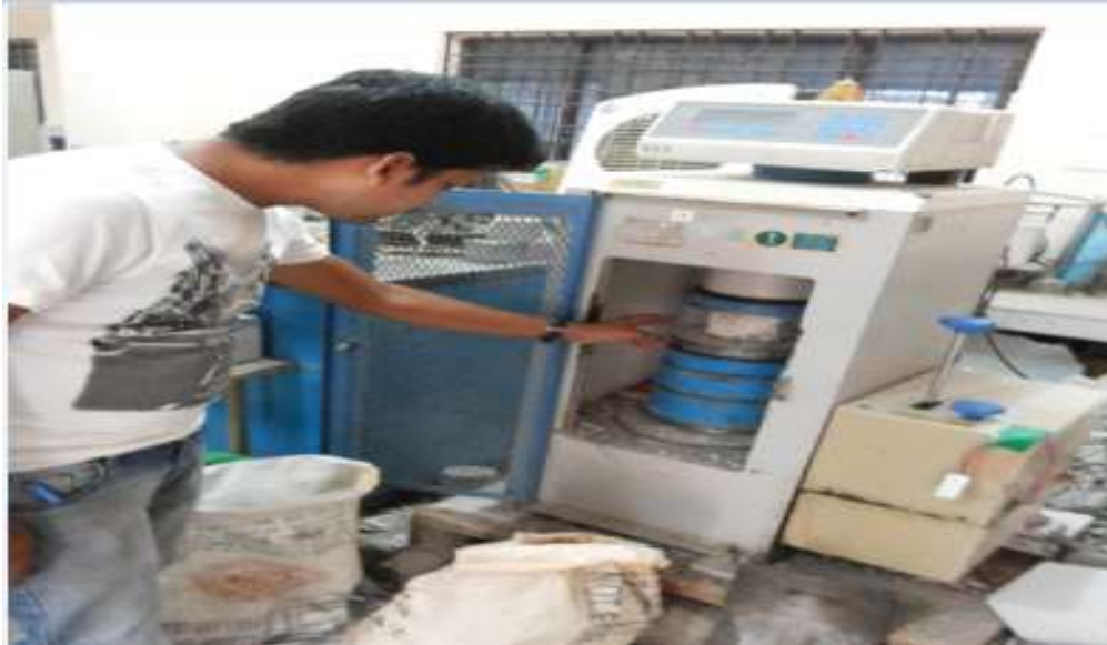
Figure 3: Compressive Strength Test Setup in CTM
