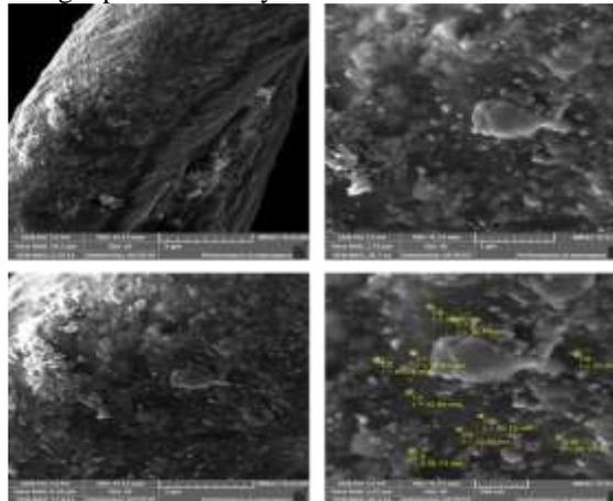
**Figure 4:** SEM of modified fabric with Alovera at magnification (5 $\mu\text{m}$ , 1 $\mu\text{m}$ , 2 $\mu\text{m}$ , 500nm)
