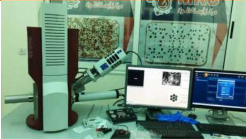
**Figure 1:** SEM and EDS Instrument
