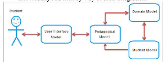
Figure 1: Typical ITS architecture
