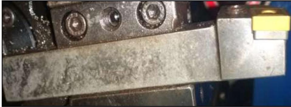
FIGURE.1 CNMG120408 insert (PVD) with Tool holder PCLNR 2525 M12
