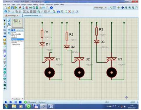
Fig.3. The scheme for starting a DC motor with a non-contact device.
