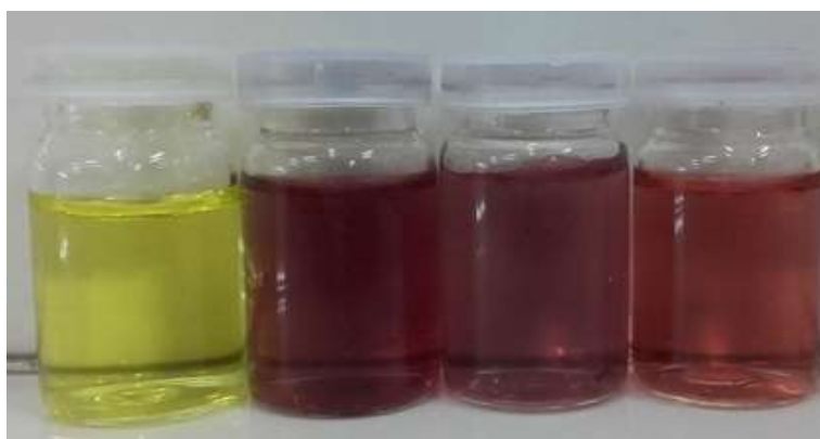
Fig. 1: Change in color from yellow to pinkish violet confirming the formation of Lallemantia royleana -Gold nanoparticles ( LR -AuNPs)
