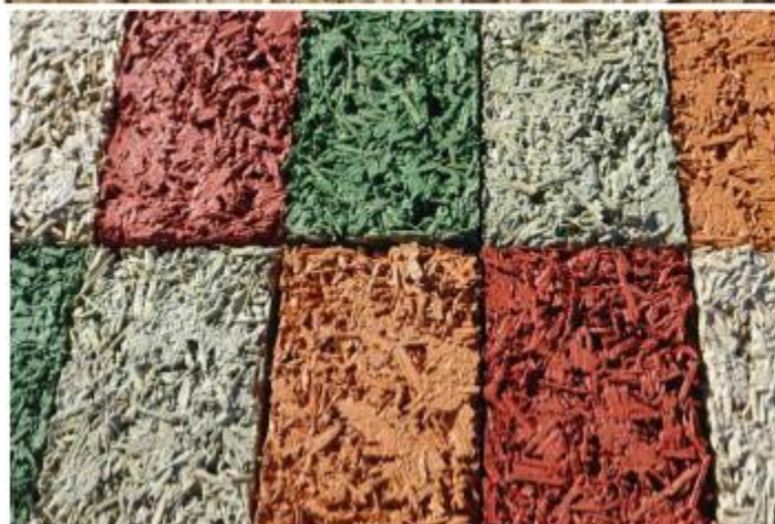
Figure 3. Natural and tinted hempcrete specimen
