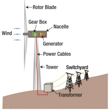
Fig.2. Layout form of a wind generator for the population
