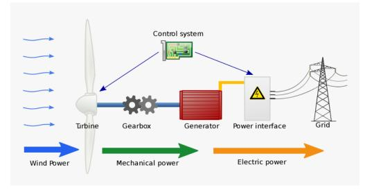
Fig.1.The principle of operation of the wind generator
