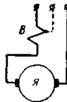
Fig. 2. Diagram of a universal engine.
