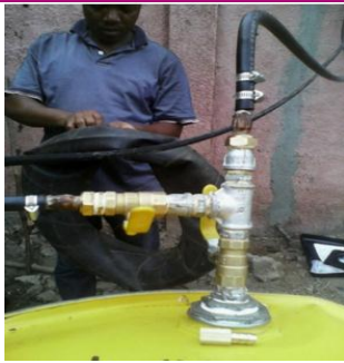
a) Fixing the air chamber
