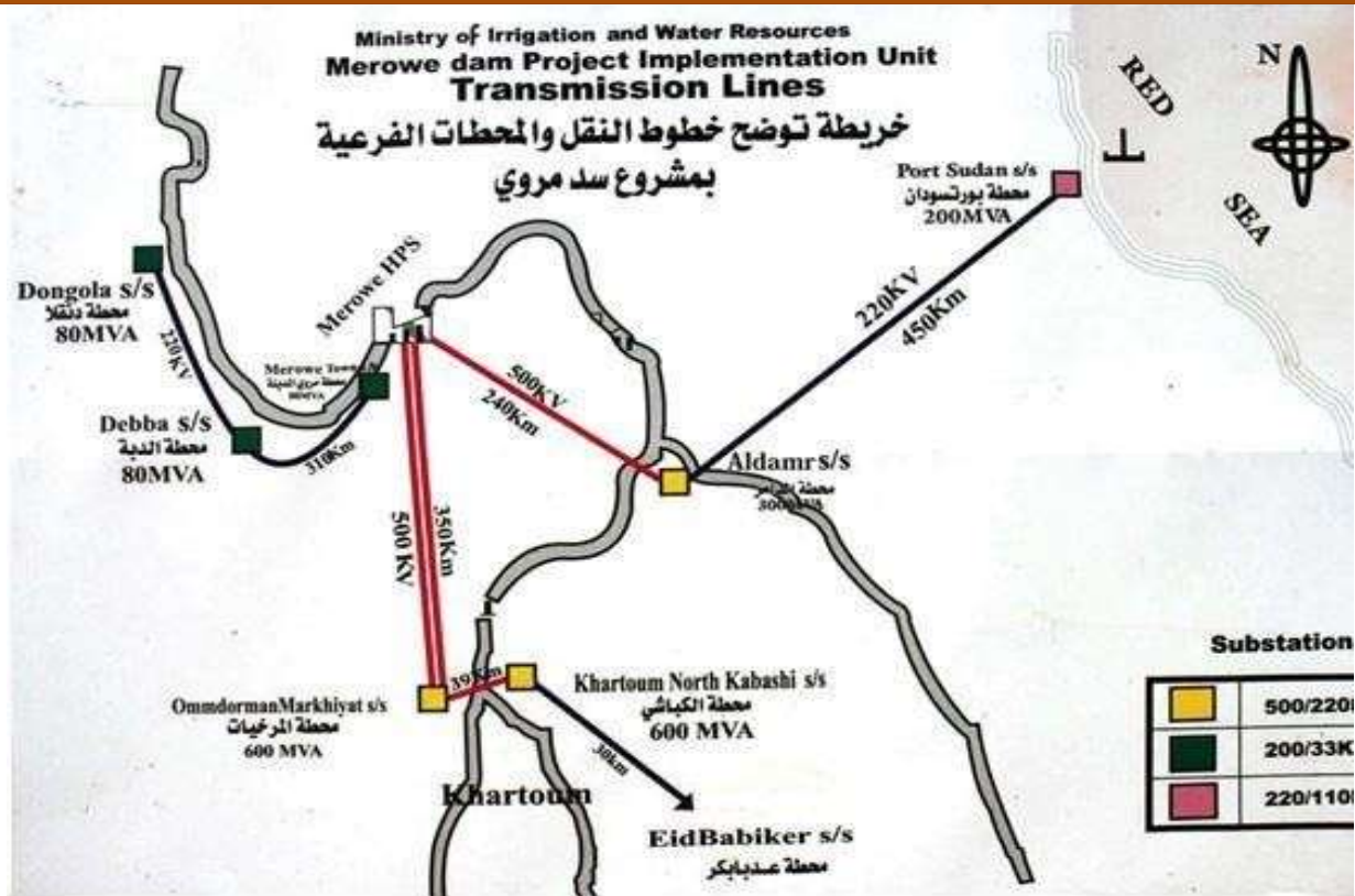
Figure 2: shows the transmission line from Meroe Dam
