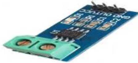
Figure 4: showing ACS712 current sensor
