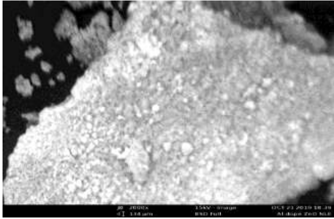
Fig. 7 SEM image of Al-doped ZnO Nps synthesized with neem leaf extract.
