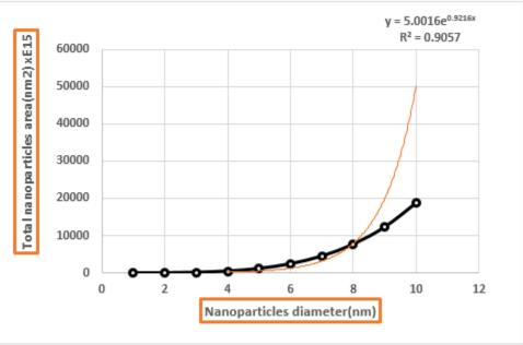
Figure 1. Exponential plots of Gold nanoparticle diameters against the total exposed area.
