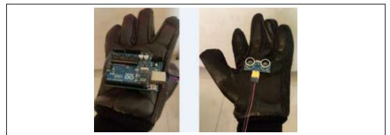
Fig. 1. Ultrasonic sensor in hand glove
