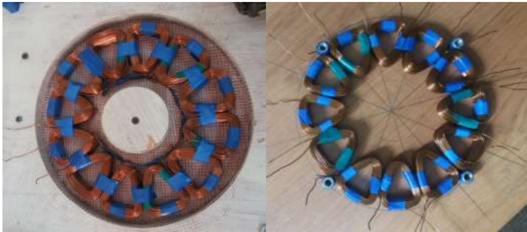
Pic.3. Generator stator winding
