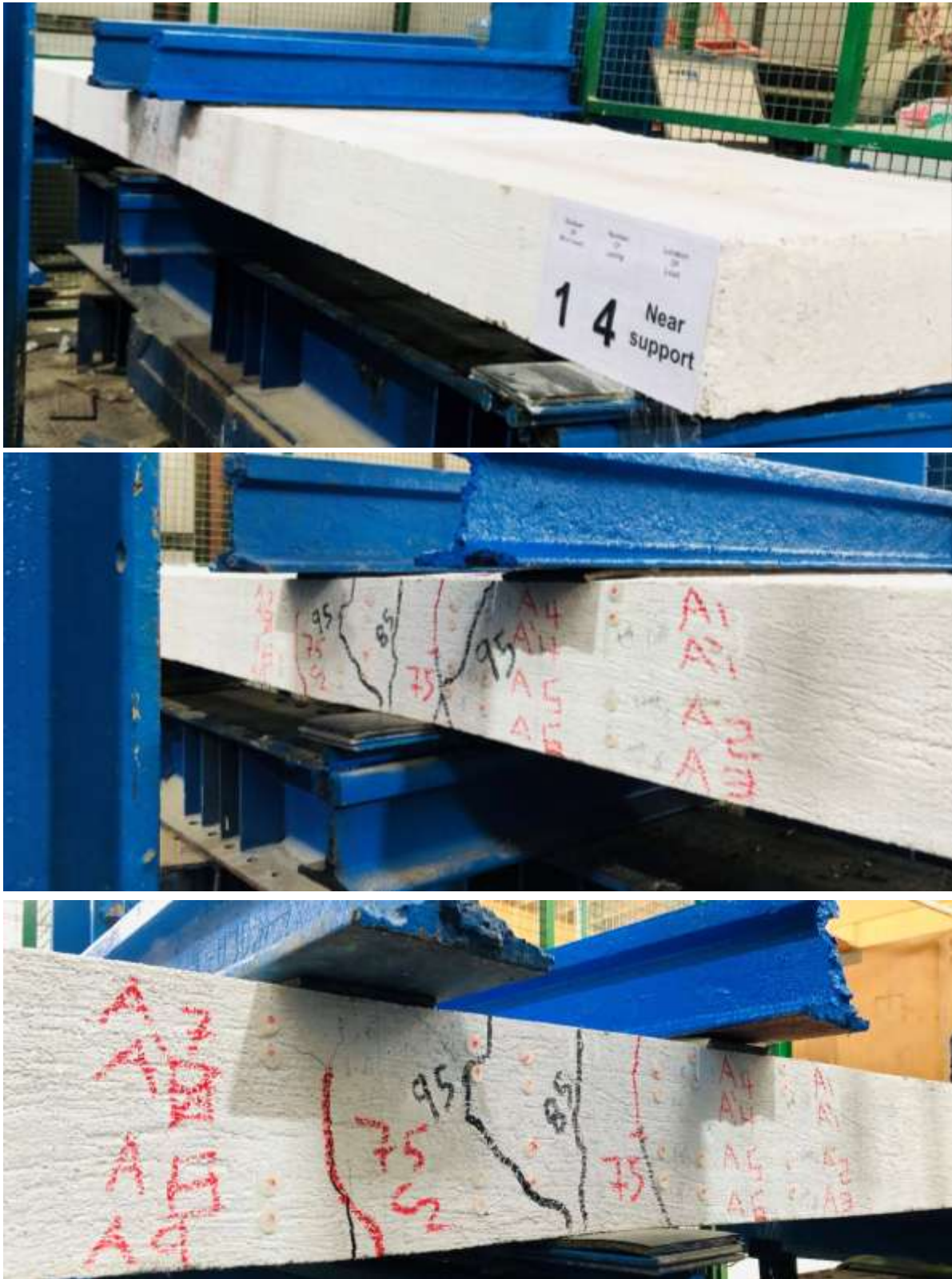
Plate 2. Failure pattern of sample MS-2'.
