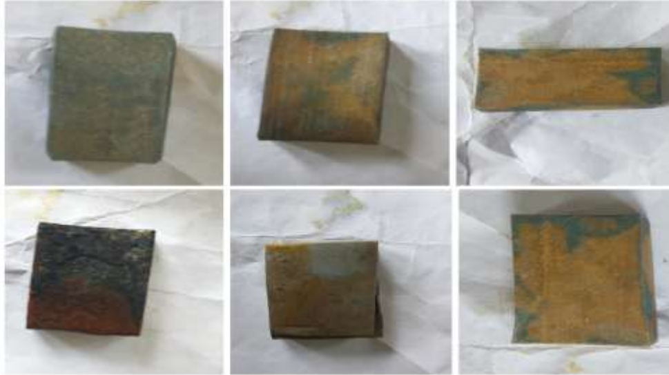
Plate 1: Coupons Used for the Test
