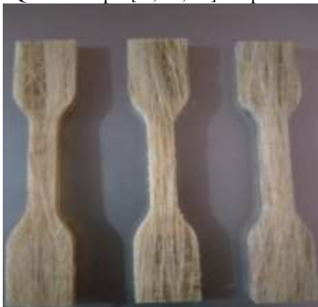
Figure 7: Tensile test specimen.
