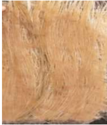
Figure 3: Quasi isotropic [0°,90°,45°] sample.
