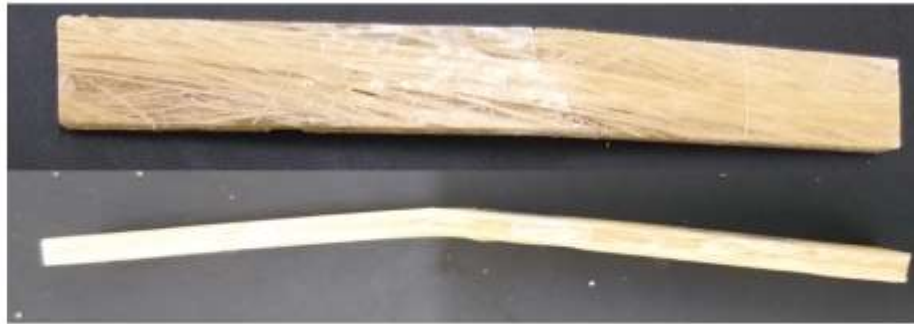
Figure (24): flexural specimens after failure.
