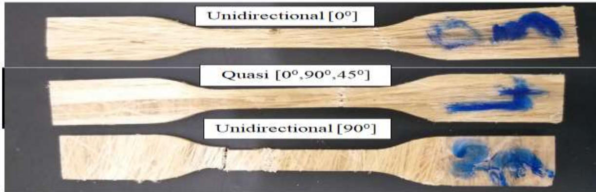
Figure (16): Tensile specimens after failure.
