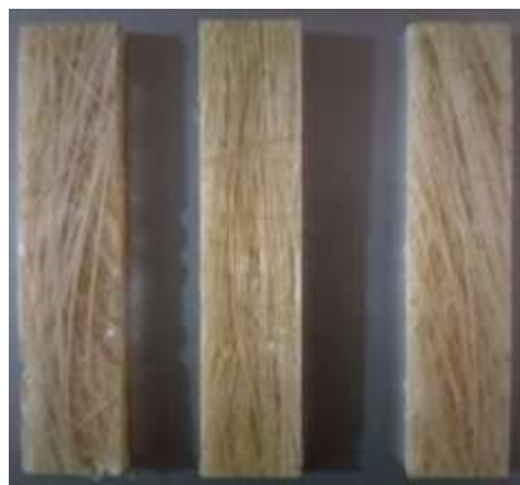
Figure 8: Flexural test specimen.
