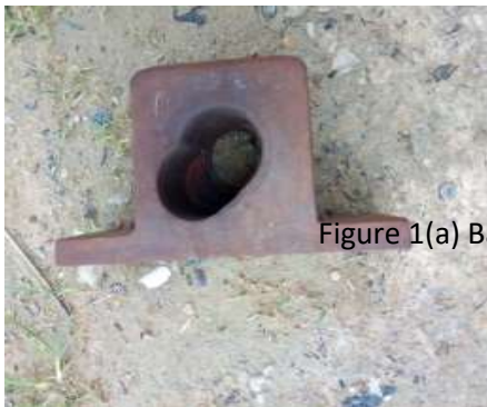
Plate: (1a) Worn Bearing Housing
