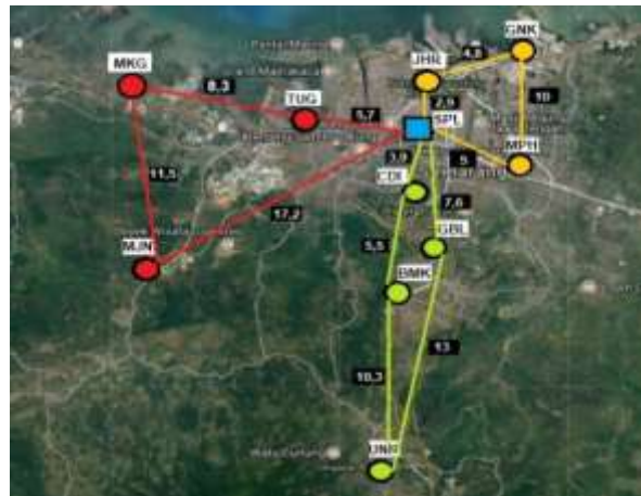
Figure 13. Results of the design of Metro Ethernet topology in the city of Semarang.
