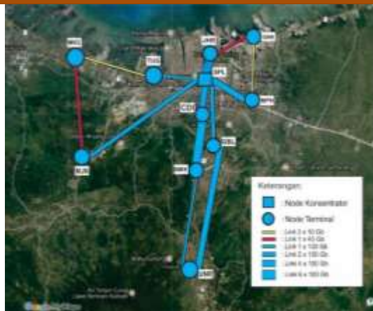
Figure 16. Results of planning for the Metro Ethernet network in Semarang City in 2028.
