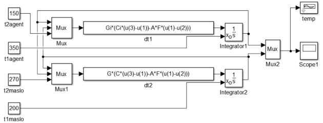
Fig. 2 Computer model of process of evaporation of cottonseed oil.
