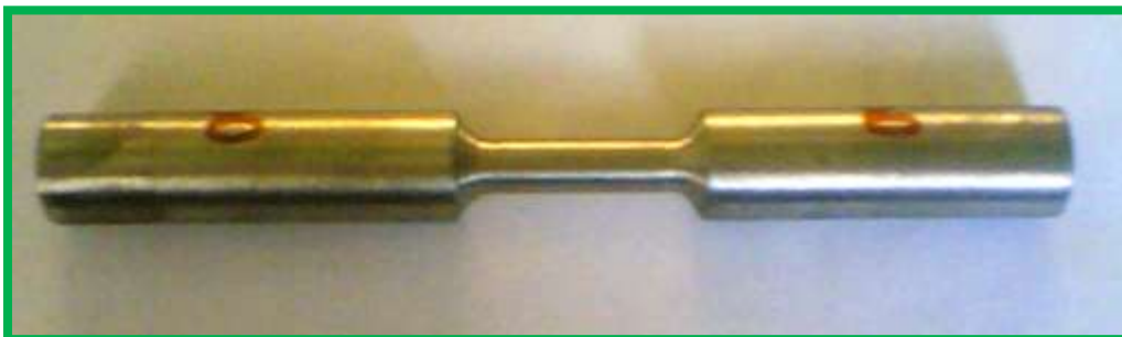
Fig. 1 Shape of tensile sample used in this work.
