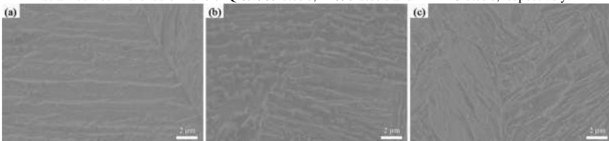
Fig. 8. Microstructure characterization of fusion zone in the small tensile specimen after tensile test. (a), (b) and (c) depicts the microstructure of fusion zone in spot welds of Q&P980 steels, DP590 steels and 22MnB5 steels, respectively. As for DP590 steels shown in Fig. 9(b), shallow dimples are displayed in the zone, suggesting the failure behavior of cleavage fractures. This result indicates the insufficient plastic deformation with a comparison to the fusion zone of Q&P980 steels. In the case of 22MnB5 steels as depicted in Fig. 9(c), the dimples are not obvious and the fracture mode is determined as brittle failure. This phenomenon could be explained by the microstructure evolution during tensile test. The martensite deformation during tensile tests (as illustrated in Fig. 8(a) and (b)), attribute to the plastic deformation during tensile tests, leading to the formation of ductile failure in the fusion zone of Q&P980 steels and DP590 steels.
