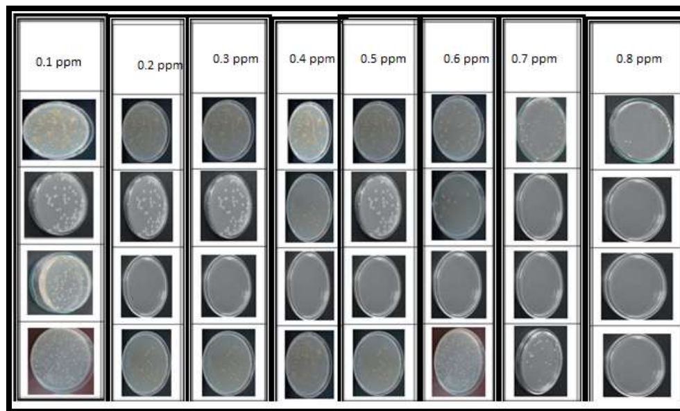
Fig (3) effect of TiO 2 nanoparticles different concentration from 0.1 ppm to 0.8 ppm on the survival of Number of viable cells Escherichia coli (CFU/ml) for 4 Weeks on the water
