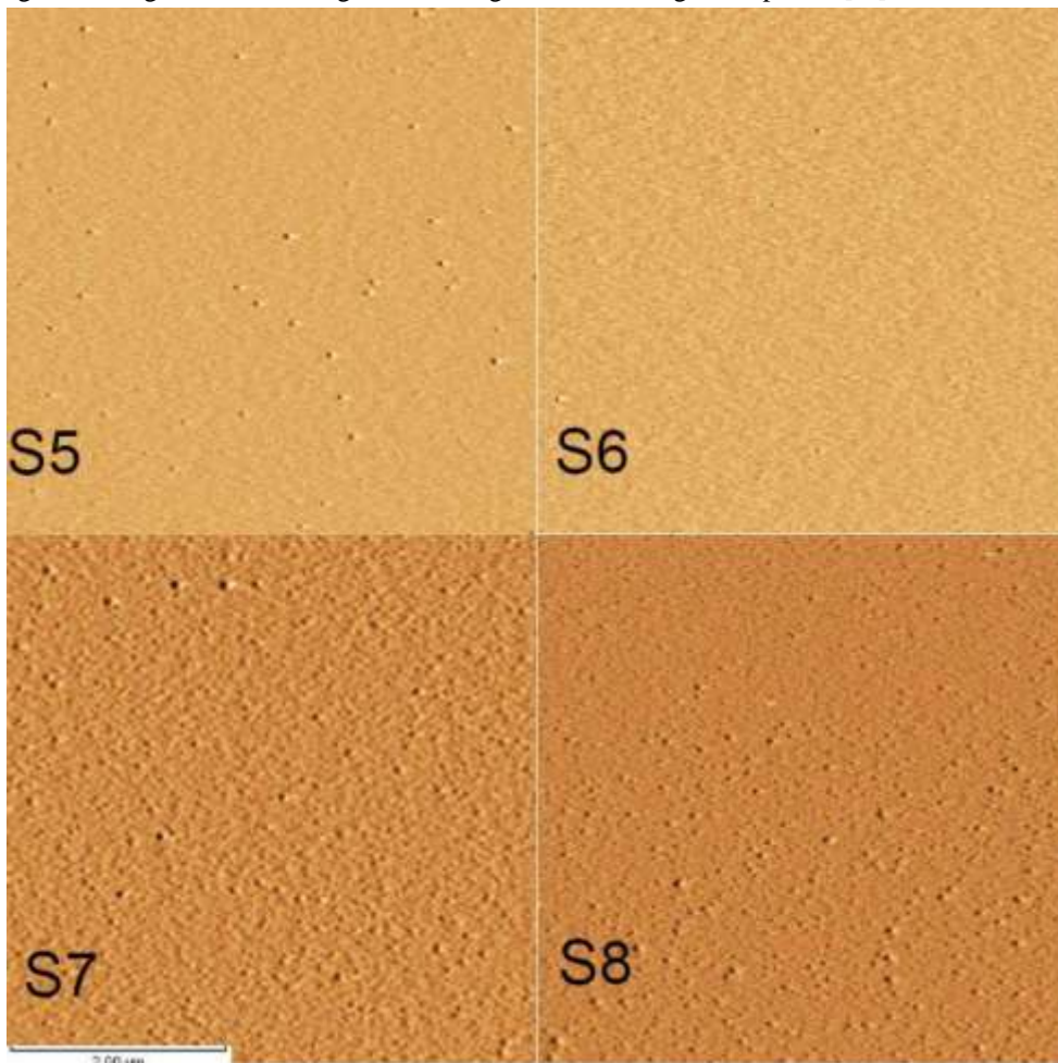
Fig. 3. AFM images of the Sn thin films deposited under different pressures and powers.
