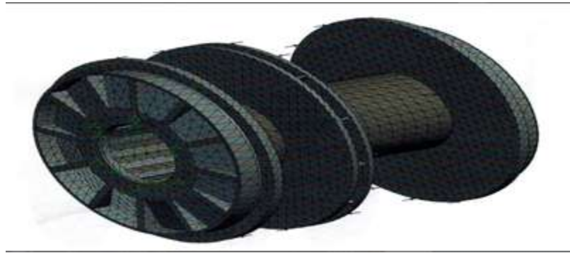
Fig. 13 New Large Diameter Split Drum Winch Structure Design FEA Shown at Hydraulic Motor Drive End
