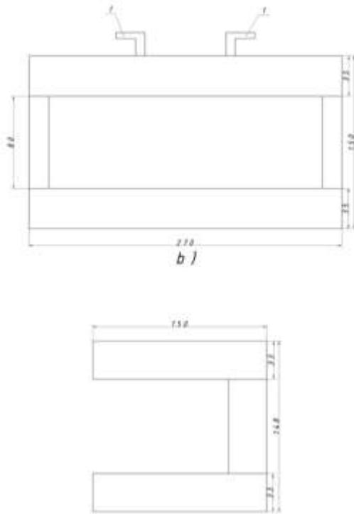
The scheme of central and side frame is given in the picture 2: a) middle frame; b) P-shaped side frames
