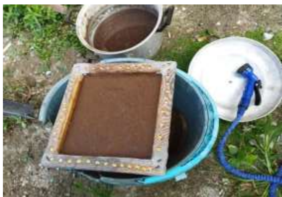
Step 7: Get a sieve or a mold and deckle, basin or any tub and put a ratio of 1:1 of the fiber and water. Start sieving your fabric for the mask.
