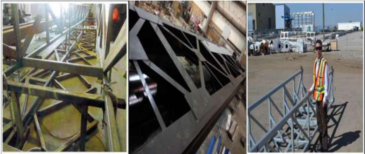
Fig.13: Rig Mast Structure Manufacturing Recommended Practices with Jigs, Template Support, Reinforcement, Bracing/Gusset, and OA&OC
