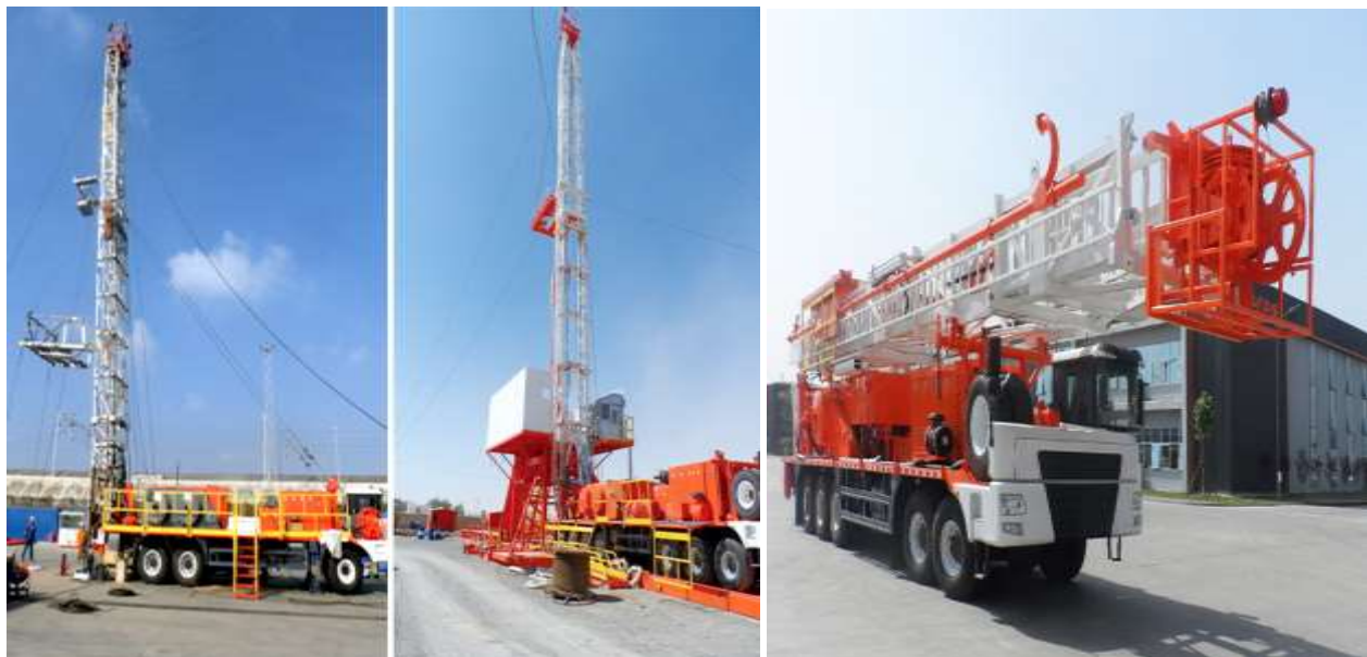
Fig.8: Jereh Truck/Trailer Mounted Workover Rig
