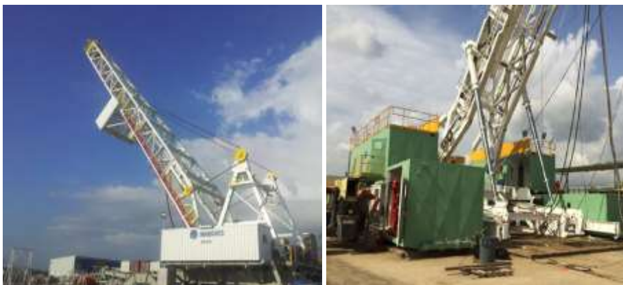
Fig.5: Left, the Mast Raised by using the Drawwork and Right, Mast Raised by Hydraulic Cylinders [5]
