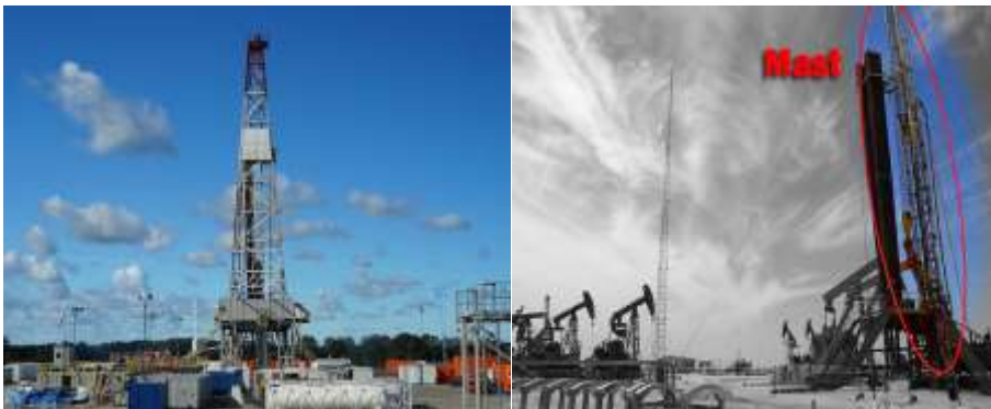
Fig.4: Onshore Land Drilling Rig Mast Structures [4]
