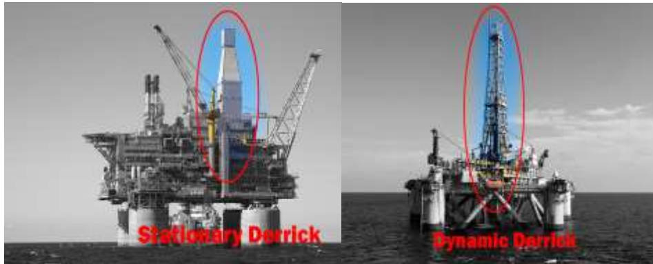
Fig.3: Stationary Derrick and Dynamic Derrick [4]
