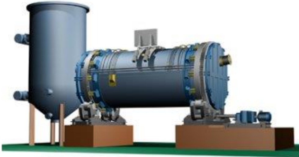
Fire refining furnace
