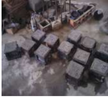
Plate 2.1: It shows the cast concrete cubes, well dressed and labeled with a standard dimension of 150*150*150mm. after proper compaction using a vibrating table or compacting rod to compact the concrete in 3 layers. Each layer requires 25 blows.
